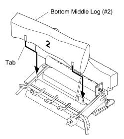
Figure 17 - Installing Bottom Middle Log
